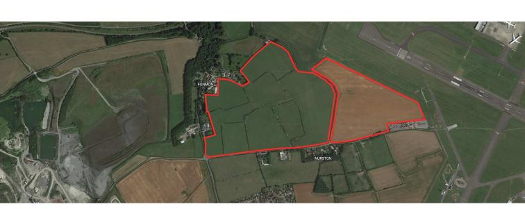
East Aberthaw Solar consists of a ground mounted photovoltaic solar farm with an electrical generating capacity of approximately 35MW together with associated equipment, infrastructure and ancillary works. The site extends to approximately 40 hectares (ha) / 98 acres in size.
